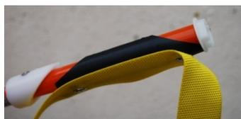
3. Make sure that the webbing is not twisted and slide the long black plastic clips attached to it on to the frame (below the white collars) each side
