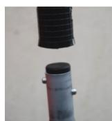
7. Fit the handle and telescopic extension, ensuring that all locating lugs are fully engaged. To adjust the telescopic extension unscrew the black plastic collar, slide the inner pole to the required position and then re-secure the collar
