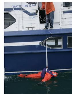
5. Recover the casualty by manually hauling on the line or by use of an appropriate winch. If required the line may be led through a davit
