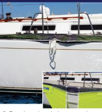
For short-handed crews - the SOS Recovery Ladder now has its own 'sock' for attachment to the toe rail, ready to be deployed at a moment's notice.
